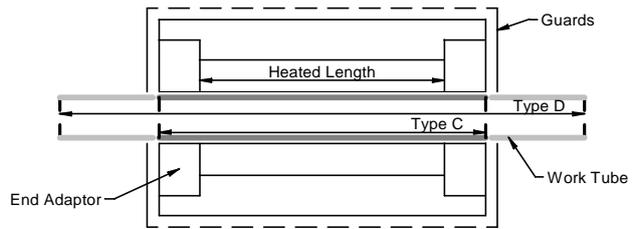
To insert a work tube it is often convenient to use a long pole (such as a broom handle) to guide it into the far end of the furnace.
