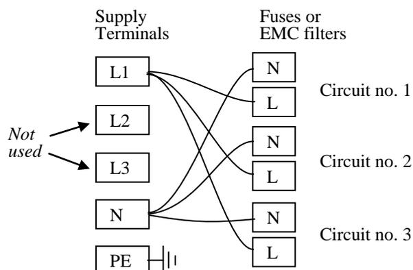
A model made to this diagram can be converted by the customer between the following supply voltages:
