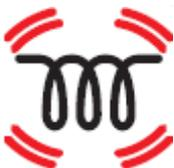
Heat Light: the adjacent light glows or flashes to indicate that power is being supplied to the elements
